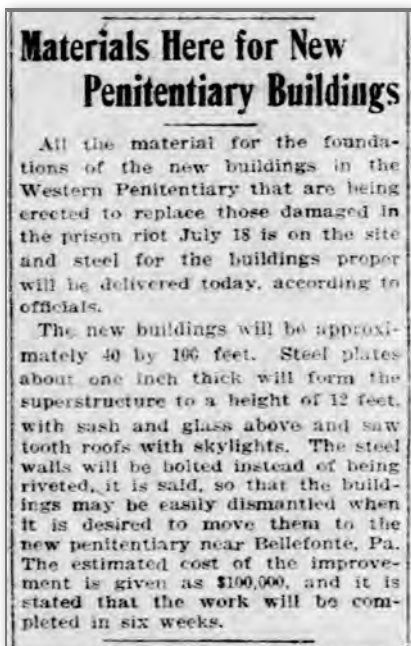
Figure 37. A Pittsburgh Post-Gazette article from October 11, 1921 discusses construction of the new buildings (albeit with inaccurate dimensions) and how they will be bolted together rather than riveted for future disassembly and relocation.
